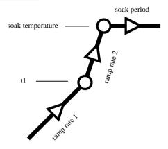
The ST312 firing segment comprises 2 ramps followed by a soak period. This single segment can be used for simple firing (biscuit firing for example).
