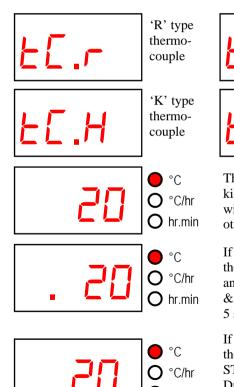
The final display should show the kiln temperature (20°C shown here) with the "C" indicator on. All other lamps should be off.
